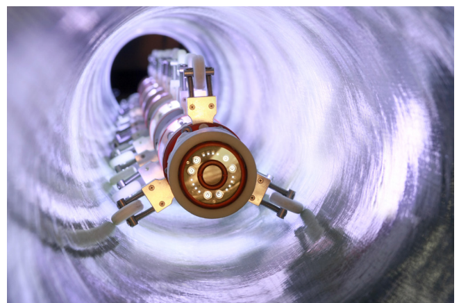
UV light source in the Berolina-Liner (DN 300)
